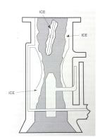
the carburetor creates a low pressure and super cooling of the metal carb body. Water vapor in
